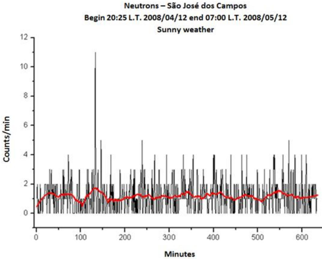
*Measurements of neutrons in ITA during clear day and dry weather on 04/12/2008. Red line is smoothed in 1 hour*
