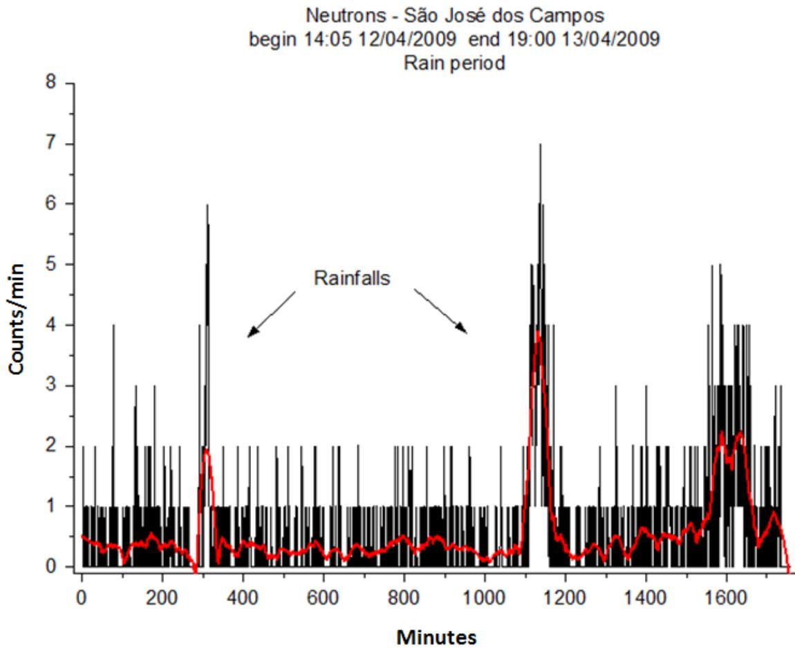
*Measurements of neutrons in rain period in April of 2009 in ITA*
