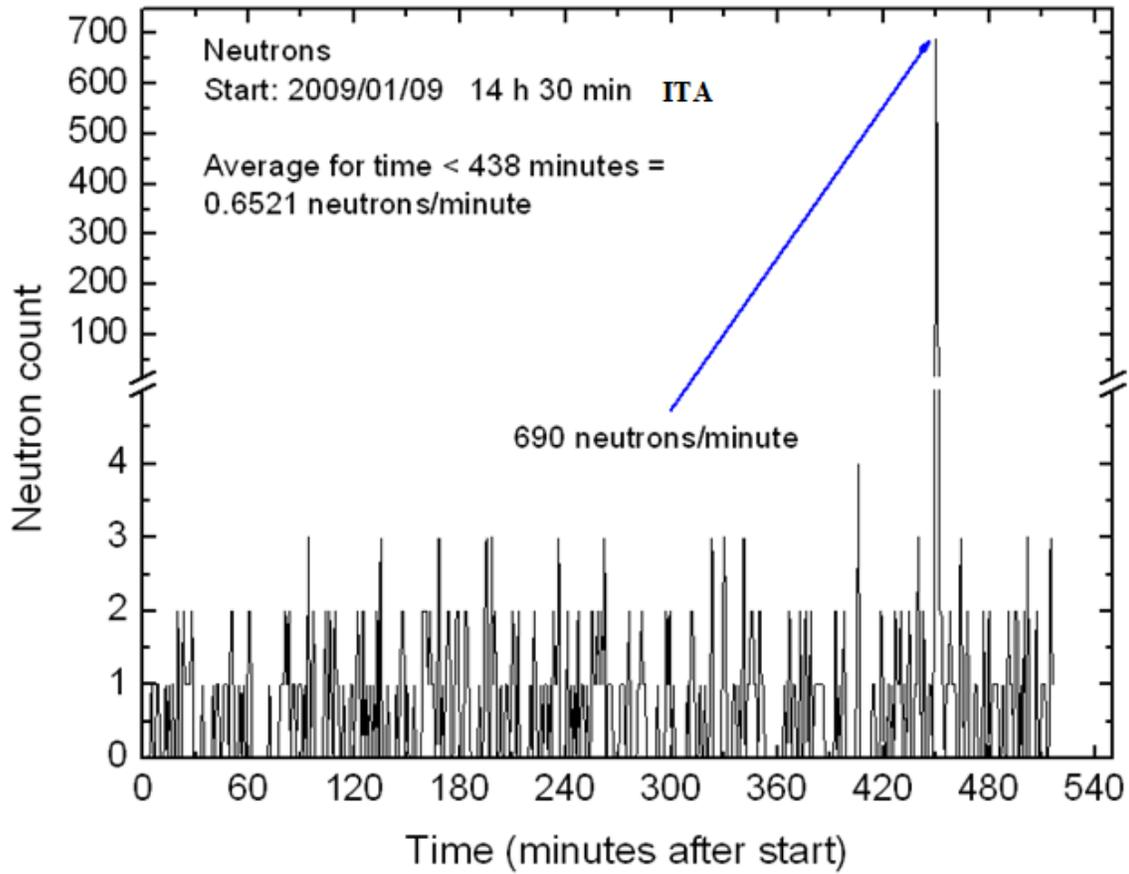
*Atmospheric neutrons produced and observed in ITA during lightning's in region [7].*
